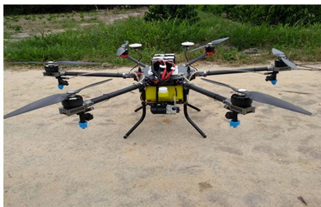
**Figure 1:** Multirotor unmanned aerial vehicle used in the spraying experiment.
